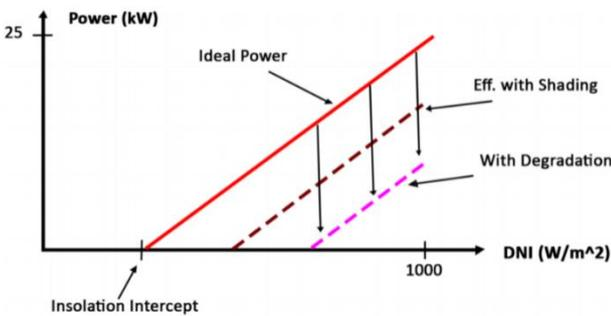
Fig. 7. Impact of shading and shading degradation factor on the system performance curve.
