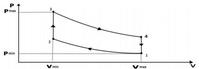
(a) Ideal Stirling cycle pressure vs volume ( $p-v$ ) diagram
