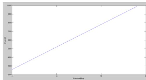
**Fig. 12.** Output power of a Stirling engine as a function of pressure.
