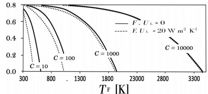
Fig. 4. The thermal efficiency of a receiver  $\eta_{th}$  as a function of the fluid temperature  $TF$  and the concentration factor  $C$ .
