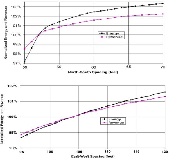
Fig. 8. Effect on revenue and energy production of variations in the north-south and east-west dish spacing.
