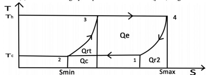
(b) Ideal Stirling cycle temperature entropy ( $T-s$ ) diagram
