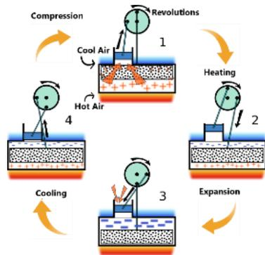
Fig. 3. Stirling cycle.
