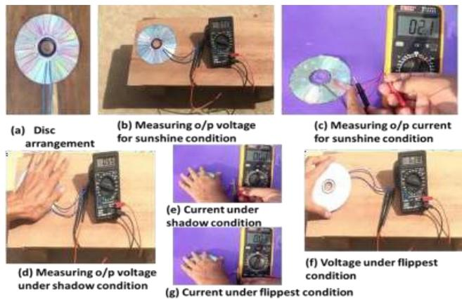
**Fig.10.** Dish Stirling prototype model: different parts and their output quantities. (a) Disc arrangement, output voltage and current measurement under (b)&(c) sunshine condition, (d)&(e) shadow condition and (f) and (g) flippest condition.
