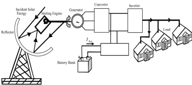
Fig. 5. Schematic diagram of the dish system.
