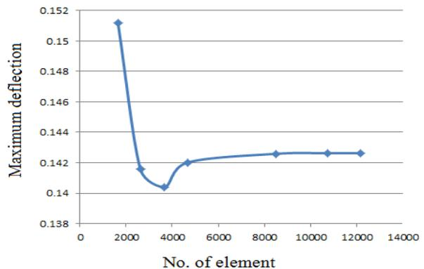
**Fig.3.** Convergence test for Shore Pile.
