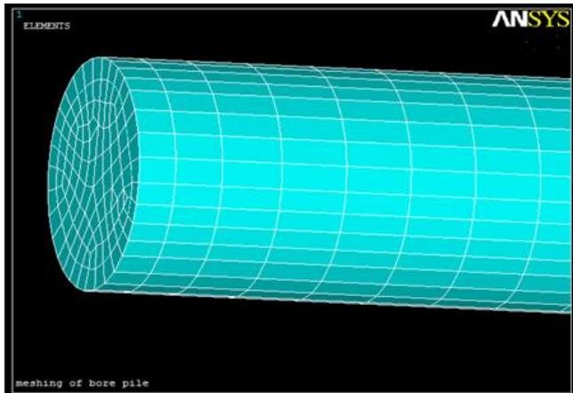
Fig. 4. Meshed shore pile.
