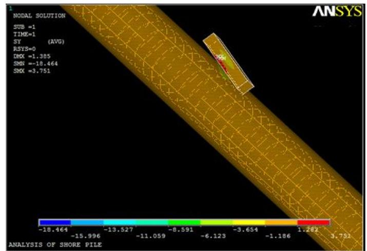
Fig. 6. Flexural stress on the Shore pile.
