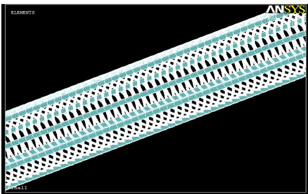
Fig. 5. Reinforcement in Shore pile.
