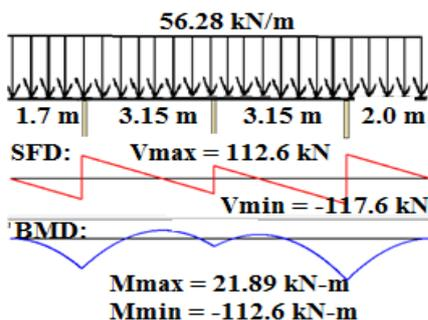
**Fig. 1.** SFD and BMD of Shore Pile obtained from Moment Distribution Method.
