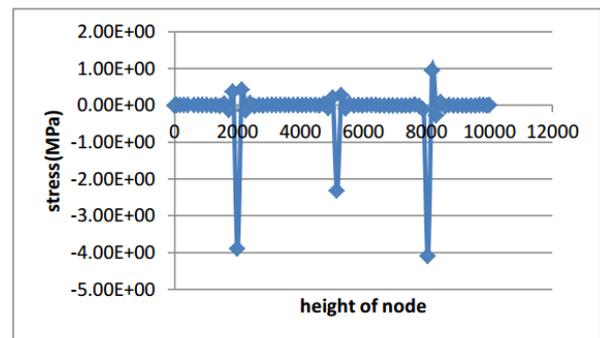
Fig.7. Flexural stress variation on the Shore Pile.
